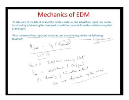
So, we have 2 modify the equation quite a bit and the rate of heat input per unit area, per unit time would then be given by the equation the total heat h total, which comes from the spark in to the work piece minus the latent heat per gram of the material which is h m assume to be h m in this particular case, times of density, times of the volume the material which is remove which is again the volume.
