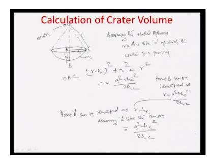
So, here let say there if the melting temperature depth is z. And the crater diameter is 2a and at r equal to 0; that means, radius equal to 0. The maximum melting temperature depth z maximum is given by h c, which is actually the crater depth for all practical purposes centimeters. And the z max off course is proportional to z h c is proportional to z.
