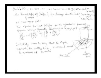
We now, need to assume certain things for example, let theta be temperature in degree celsius of a particular zone in that circular region t be the time in seconds, at which theta is being monitored, k be the thermal conductivity of the anode, which is also the work piece over which this melt phenomena is happening the, this can be assumed to have a unit of calorie per centimeter, second degree celsius.
