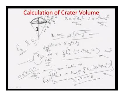
So, then it just spoils down to a simple problem of integration that is assume, this crater to be present like this just to stead the sphere of side down this gay this write here is the full depth of the crater h c. And it is a part of this is sphere here with center o and basically, we can actually consider a very small element like a cylinder in this particular area and try to see what is the volume of this and integrate such cylinders starting from the point a to the point b ok.
