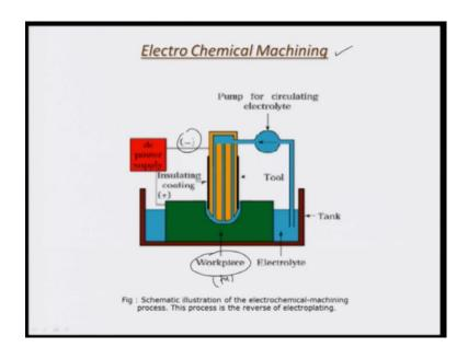
So, let us look at some potential applications and just to illustrate once more, the ECM process is about the electrochemical transport, of material from a positively charged work piece made the anode and a negatively charged tool center, in the presence of an electrolyte.
