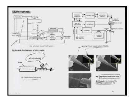
The work piece has been given small rotations and the wire cathode has been able to generate this kind of a very pin pointed shape. The EMM system that they use in this particular case, is illustrated in this figure right here, shows the power supply system for such an EMM process.
