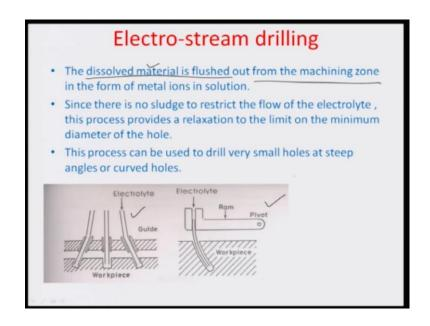
So, naturally the dissolved material is flushed out of the machining zone. You can see here are 2 illustrations where, there are steep or curved holes which are being made using the electro stream drilling. So, the dissolved material in this case is flushed out from the machining zone, by pushing it through other negatively charged stream of acid which is following.
