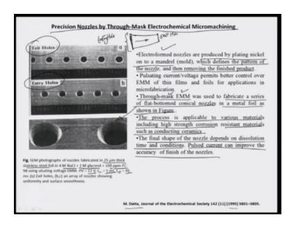
Let us look at the few more examples of what EMM electrochemical machining can do micro machining. This for example, is again borrowed from this group at all in 1995. And they talk about the fabrication of precision nozzles through a mask approach. So, they use, they develop this electroformed nozzles and they produce it by plating nickel on to a mandrel mold which defines the pattern of the nozzle and then removes remove the finish product from in.
