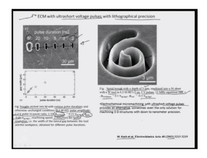
The other example that I have borrowed is from, kock at all is group which they reported in 2003, where they talk about the fabrication of various ultra short small miniaturized structures, with using ultra short voltage pulses. And they have almost claimed that, they get lithographical precision by using these ultra short voltage pulses, when they do ECM
