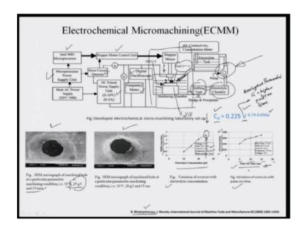
Let us look at some of the work done by many groups earlier. This shows how the ECMM unit is more controlled process than the ECM unit. Here, this region is really the region which is the machining center, you have a work piece here, and you have a tool region. Again tool is negative, work piece is positive as any other ECM process. There is a electrolyte which is being pumped through this nozzle right here, into the work piece zone. And of course, there is a flow handling system.
