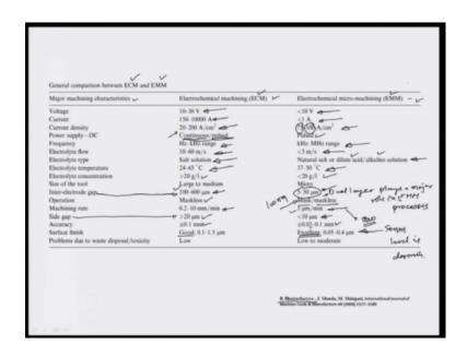
So, the first comparison that I would like to draw between ECM or ECEMM or a EWCMM process, that is, electrochemical micro machining or electrochemical machining process, is given in this table very nicely by Bhattacharya at all in 2004. And here, let us look at some of the differences in terms of the major machining characteristics, in both these processes ECM and EMM or ECEMM.
