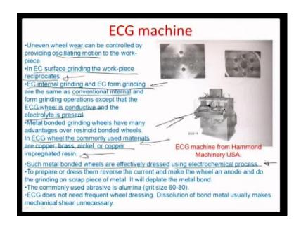
So, the EC surface grinding typically, necessitates the work piece to reciprocate with respect to the tool for example, this is a tool which is shown where you can see this is the stage here, which is containing the work piece and it has a rectilinear motion in both the x and minus x direction as the tool moves in clock or anticlock wise direction. So, in the EC internal grinding and form grinding the basic concept is same as the conventional internal and form grinding operations.
