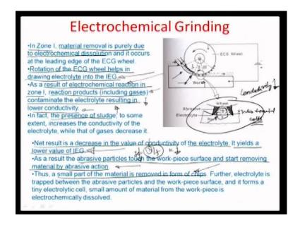
So, a the effective area in which machining is taking place can be divided into 3 zones and you can see the mark here as zone 1 2 and 3 respectively. Let see individually, what happens in all these 3 different zones in the ECG process. So, as I already illustrated before the electrochemical grinding is a combination of electrochemical dissolution as well as mechanical abrasion or removal of material mechanically there is a 9d 10 combination.
