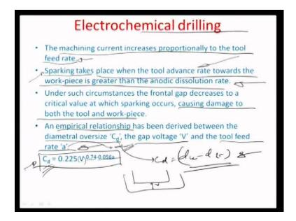
So, there are certain effects which take place particularly in electrochemical drilling process for example, 1 such undesirable effect is sparking and sparking typically takes place when the tool advance rate towards the work piece is greater than the anodic dissolution rate. So, you already know from the electrochemical machining theory that if the tool is approaching the work piece there is 1 aspect of the tool getting dissolved.
