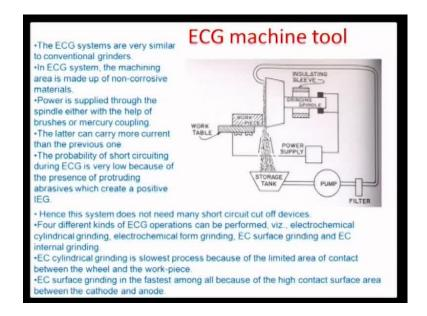
So, that is about the basic process of electrochemical grinding, there are certain other aspects associated with the machine tool as such it has to be a tool as any other normal grinding process, because there has to be relative rotation between the electrochemical wheel and the work piece surface.
