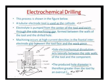
So, let us look, at these processors and to begin with we start with just electrochemical drilling operation. So, the fundamentally this processes illustrated here. So, you have a tubular electrode which is used as the cathode in this case, which is also the tool. So, this is the tool site and the electrolyte is pumped from the center of the tool and exists
