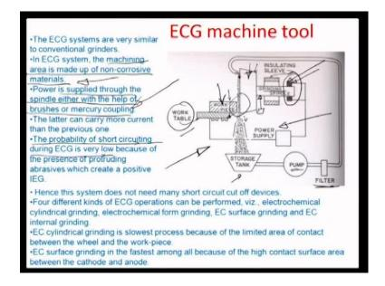
So, this slide here illustrates briefly how the electrochemical grinding machine tool would look like. So, you have a work piece here for example, and then you have a grinding spindle and this is the grinding wheel and there is a flow of electrolyte pass the
