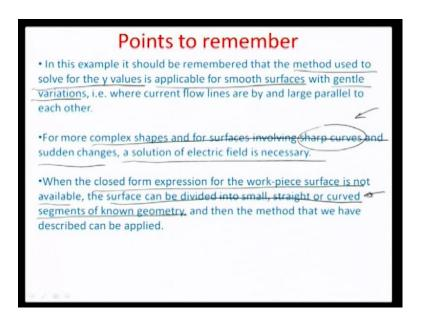
So, somehow the important points to remember particularly when we talk about this. So, called ECM process that it should be remembered that, the method used to solve for y value is typically, applicable for smooth surfaces with some gentle variations 1 of the reasons why smooth surfaces are the point of discussion here, is that if the surface is too rough then there would be a variation local variation of the electric field and in our approach that, we have used or the algorithm.
