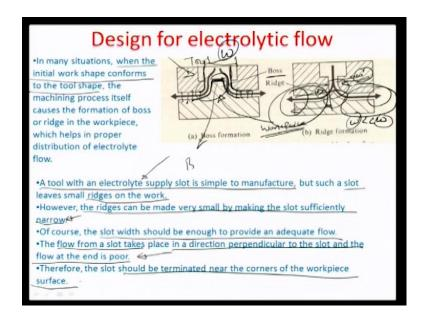
So, in many situations for example, when initial work shape confirms to the tool shape for example, in this particular case, you see that this is the tool. And there is a boss on this work piece, which has somehow coming to the path of the electrolyte flow. So, there is a small chamfered corner of this tool and there is concentric coaxial channel, which is available for the electrolyte flow. And the boss has somehow the boss in the surface
