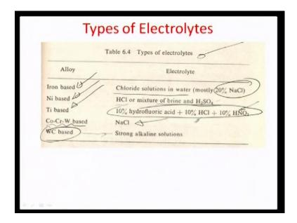
Let look let us look at some of the systems which are existing typically for some conventionally used alloys of engineering importance. So, for iron based systems the electrolyte that is normally used as chlorine solutions and water you know, brine solution comparing our consisting of kitchen salt and water 20 percent concentration is typically, used for iron based work pieces for electrochemical machining.
