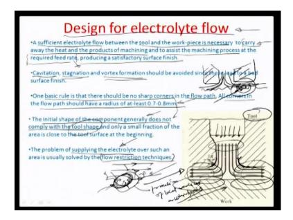
So, the other aspect I would like to really illustrate, for the ECM process is the design for electrolyte flow. So, 1 aspect we have already discussed, is how the velocity and pressure could be calculated from before the other very important method or the other very important part of the layout that, we have to plan is how you flow in the electrolyte to begin with.
