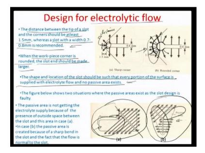
When you are designing the tools for with which sharp corners, for ECM process you have to follow some thumb rule for example, the distance between the tip of a slot and the corner. So, we are talking about this distance from this tip to the corner. There should be at least 1 point 5 m m for obvious reasons that there has to be sufficient. So, the there may be some electrochemical machining of the tooling itself although the tooling is chosen in a manner.
