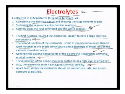
Let us now, look at the other part that is electrolytes which you need to design for ECM systems. So, let us just 1st find out what are the basic functions associated with an electrolyte. So, 1 it allows the completion of the electrical circuit between the tool and the work piece. So, this is the only conducting means between the tool and the work piece and it should allow flow of large currents.
