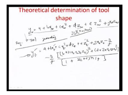
So, in case the equation of the work piece is a 3 dimensional equation. So, y w in this case is related to let say, a plus b x w plus c x w square plus some d z w. So, we are including both all the 3 coordinates here, the x y and zee. So, it is a courtesy in coordinate system d x w d z w plus e z w square plus g x w z w.
