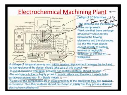
We now look at the ECM plant the way that the electrolyte is circulated and all these machining happens. So, this is a very nice schematic of what all goes into an ECM system. So, you should have a electrolyte pumping mechanism this is a electrolyte storage and basically have a pumping mechanism and a discharge mechanism. So, normal operation you can keep this valve on. So, that whatever pumps out goes in back and if it is switched off then the electrolyte can get circulated into the system.
