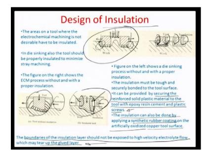
So, the other issue which is needed for Considering, ECM is how to develop good insulation on the tool and there are good number of reasons for developing insulation. For example, let say this figure here, considers a un insulated a completely non insulated tool. So, there would be ECM carried out between the tool and the work piece in this direction which is what we need or what is intended for, but then also there would be ECM carried out between the sides of the tool.
