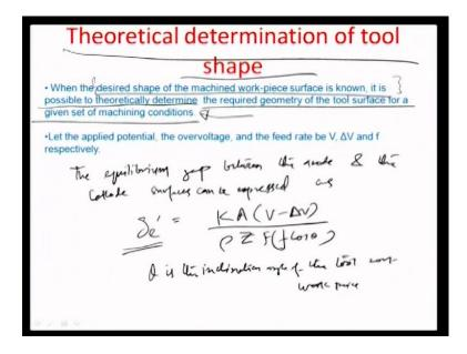
So, we will look at the 1st aspect now that is determining a tool shape so that, the desired shape of the job can be achieve for a micro machining or for a machining condition. And in that respect I would like to sort of propose theory were we want to theoretically determine what is the tool shape based on a certain function, which is ah known to be the final shape of the work-piece that we would like to generate using ECM.
