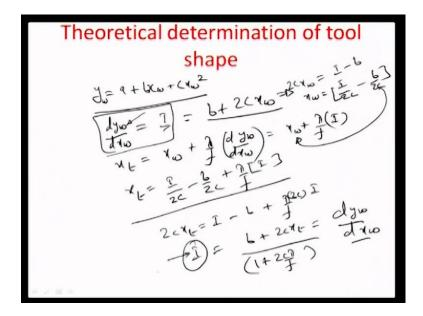
So, let suppose that there is a function y on the work piece surface which is related to x 1 the tools of tool surface by the quadratic equation a plus b xw plus c xw square. Now we want to find out how to map it from the tool of the work piece surface into the tool surface. So, you first find out what d yw by d xw is let this we equal some value I right and this is actually it can be represented as b plus twice c xw.
