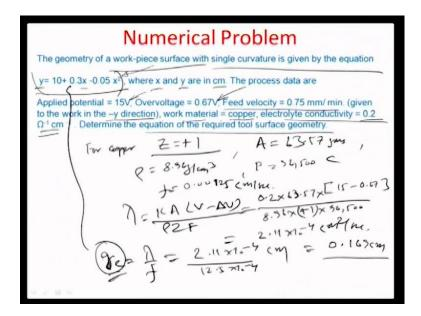
Here, as you see here the geometry of a work piece with symmetrical is given and this geometry is given by the equation y plus 10 y is equal to 10 plus 0.3 x minus 0 point 0 x square. Or you know that these are values in centimeters and the process data is that applied potentially 15 volts over voltage which is needed is 0.67 volts.
