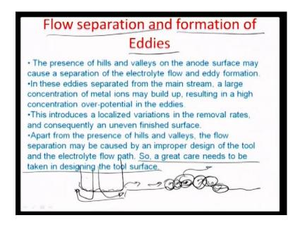
The other important factor which is a responsible for the creation of surface roughness is the formulation of Eddies and separation of the flow. If supposing there is a rough surface which has been created, because of the selective dissolution of the field due to an electric electro chemical tool, it is always proper to assume that there may be a case local circulation. But it will only when the electrolyte is flown in both the directions like this.
