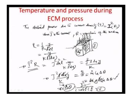
So, now we would somehow like to find out relationship between the current density which is the main reason for the heat transfer, from the tool or the work piece on to the electrolyte. And if you look at that the electrical power due to the current density which is dependent on the flow of the ions right is equal to j square i square r, where i is the current and r is the resistance of the medium.
