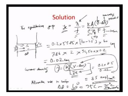
So, let us look at how we step by step solve such a design problem. So, the equilibrium gap y e is of course, given by lambda by f for the constant feed case as you may remember in the section on kinematics and dynamics of ECM. And this can further be represented as k, conductivity of the electrolyte times of atomic weight of the species that you are dissolving which in this case is pure iron.
