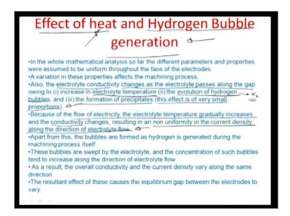
Let us look at some of the other important corollaries of an ECM process. There are several problems associated when particularly talk about electrolysis. So, the more important aspects of associated with the electrolysis are this: hydrogen bubble generation thereby changing of local conductivity or thereby registering a change in local conductivity and heating; non uniform heating of the electrolyte while passing through the equilibrium gap.
