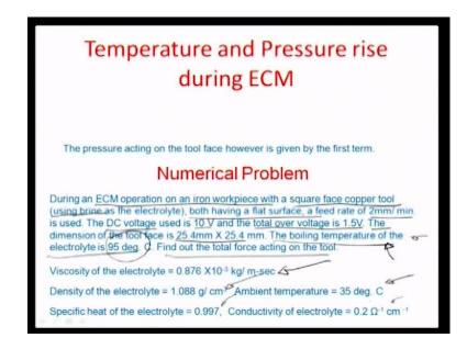
So, let us now try to solve numerical problem that, during an ECM operation on an iron work piece with a square face copper tool using of course, salt water solution or brine as a electrolyte. Both having a flat surface to begin with and a feed rate of about 2 millimeters per minute, the d c voltage that is used is about ten volts and the total over voltage is about 1.5 volts. The dimension of the tool face in this particular case is it is a square tool.
