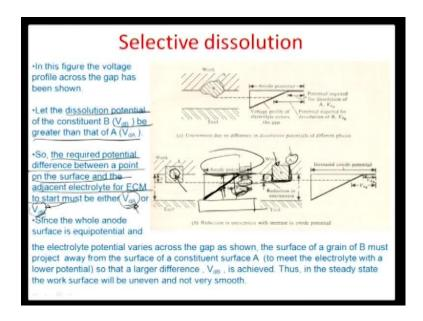
So, if we assume that the dissolution potential of b v d b id greater than that of a v d a. So, the required potential difference between a point on the surface and the adjacent electrolyte for ECM to start, for the face a must be v d a or must be v d b for the face b.
