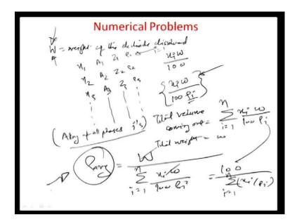
So, what is rho average and how do we determine it? So, the average density can be really found out by looking at, what is the total weight which is involved. So, let us say if w is the total weight of the electrode that is dissolved. And this w has components x1 x2 x 3 so on so forth percentagewise of materials with atomic weight A1 A2 A3 so on so forth with a valency states, the lowest valency state Z1 Z2 Z3 so on so forth.
