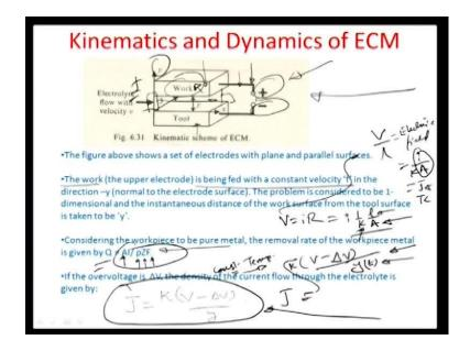
The flow of the electrolyte happens at a velocity V, from this end right here to this end. So, the flow is in this direction of the electrolyte. And we want to model how this system works because there would be a dissolution component associated with the work piece and there would be a relative motion between the work piece and tool. And so there should be some kinematics taking place between this dissolution which is receding away a surface and the approach of thee work piece towards the tool.
