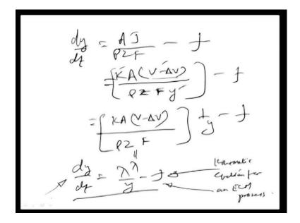
So, we can say that dy by dt equal to AJ by rho zF minus f can be written down as KA times of V minus delta v divided by rho zF. Where this KV minus delta v by y is the current density vector minus f, if you pull out y of the whole term happens to be some constant times of 1 by y minus f, let us call this lambda. So, we have dy by dt is equal to lambda by y minus f and this is actually the kinematic equation for an ECM process.
