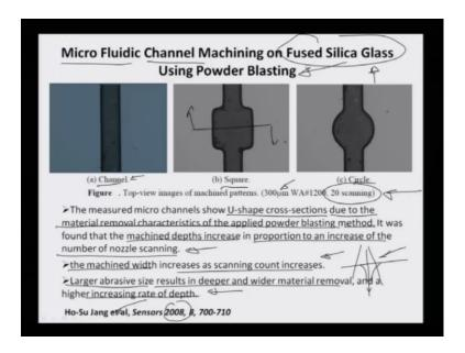
This for example, is other very powerful powder blasting techniques, is same as abrasive jet machining in different manner. And here it is used for carving out micro fluidic channels on fused silica glass again one thing, which is observable here is the most of the
