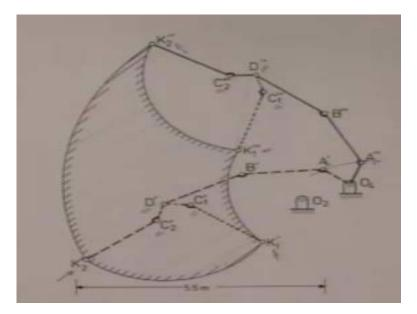
If we look carefully at the original diagram, what we can see, that this distance  $O_4A$  never changes because they belong to the same rigid body. Consequently A lies on a circle with  $O_4$  as center and  $O_4A$  as its radius. The maximum distance between  $O_2$  and A, which is given to us, locates this point. Minimum distance between  $O_2$  and A, which is again specified in the problem locates this point.
