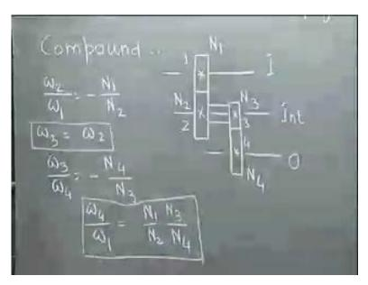
Now, let me discuss how to analyze compound gear train and what is a compound gear train? Let me now discuss what we mean by a compound gear train. In a compound gear train, there will be more than one gear on some shaft, either on the input shaft or output shaft or intermediate shaft, there must be one shaft in this transmission. In this gear train there will be more than one gear on one shaft.
