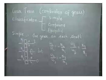
Gear train classification: gear trains are normally classified under three headings- namely, simple compound and epicyclic. These are the three normal forms of gear trains. Simple gear train is that gear train, where on each shaft there is only one gear. There is input shaft, there is output shaft and there maybe several or one intermediate shaft connecting the input to the output shaft, but on each shaft there is only one gear. So, simple gear train has one gear on each shaft.
