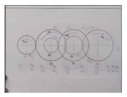
This figure shows again a compound gear train. As we see, on these two shafts there is more than one gear, there are two gears one here and one here. So this gear is connected to this gear, on the same shaft there is this gear which connects to this gear and on the same shaft there is another gear which is connected to this gear. So from here to here, the speed rotation is being transmitted, these two are intermediate shafts. So, this is a compound gear train.
