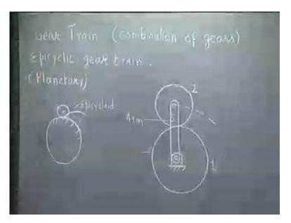
Whereas in epicyclic gear train, we will see that there will be one gear whose axis is not fixed in space, because the gear is mounted on an arm and that arm is rotating and carrying the shaft of that gear along with this. In such gear train, if there is one such gear, we call it an epicyclic gear train. Some books call it planetary gear train. To show, suppose I have one gear here and another gear there. This gear, let me call it 1 and this gear number 2, but gear number 2 is carried by this
