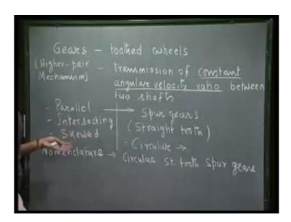
Today, we start discussion on a new type of higher pair mechanism, which are very commonly used and I am sure all of you must have seen this mechanism which are called gears; gears are nothing but as you know that toothed wheels; these are used all over machines to transmit constant angular velocity ratio between two shafts.
