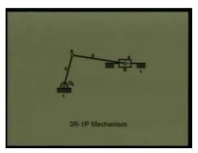
In the previous mechanism, the fixed link had a revolute pair at one end and a prismatic pair at the other end.
