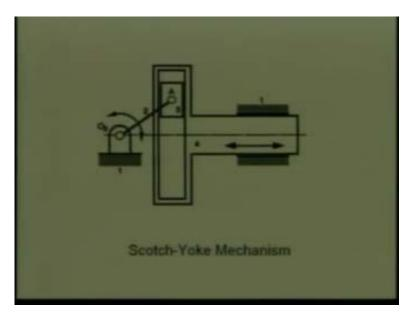
However, the to and fro rectilinear oscillation of the piston of a slider in a slider crank mechanism is periodic, but not purely harmonic. This periodic motion tends to be harmonic as the ratio of the connecting rod length to the crank radius keeps on increasing.
