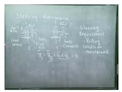
Let us say, this is the front view of the one of the wheels, front wheel's front view. As we see, the front wheel is normally mounted on a short axle which is pivoted to chassis and the pivot axis can be vertical, this is the body of the automobile and this is the pivot axis. When car wants to take a turn, it is this front wheel, rotates about this pivot axis. There are other types of steering mechanisms, where this pivot axis may not be vertical, it is
