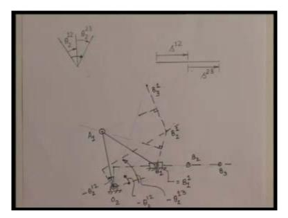
Let me now say, this design of this slider crank mechanism to generate these two pairs of coordinated movement as we have seen in the previous problem. It is the same problem, only thing is we solve it a little differently by assuming the crank pin location arbitrarily which we call it as  $O_2$ . We assume the other moving hinge which is connecting to the slider at the first position is here which I call it as  $B_1$ .
