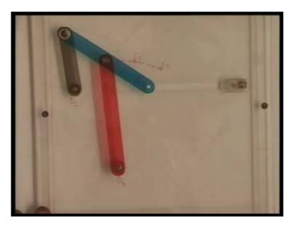
For that purpose, we remove this slider and take this fourth link and put a hinge between those midpoints of the original connecting rod connected by this rigid link whose center is at  $O_4$ , which is hinge at  $O_4$ . This is the other fixed link. We have got a 4R linkage namely,  $O_2$ , A, B,  $O_4$ . This is designed from the previous slider crank, only the slider has been removed.
