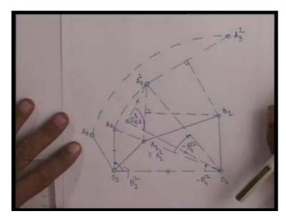
To do this we proceed as follows. Let me now first choose the fixed hinges  $O_2$  and  $O_4$  arbitrarily. This is  $O_2$  and this is  $O_4$ . We also choose the first position of the crank pin A
