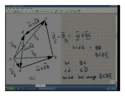
We go back to the velocity diagram we again have bc, de and let us see the ratio of these sides of these two quadrilaterals in the velocity diagram, in the acceleration diagram. Small bc is the omega cross BC, small cd is omega cross capital CD, small de is omega cross capital DE and eb is omega cross capital EB. Thus, this quadrilateral bcde is nothing but a scale drawing of the
