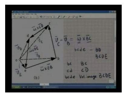
Like in the velocity diagram, this small bcde is the velocity image of capital BCDE. This is the concept of velocity and acceleration image and we shall see its utility in a later example.
