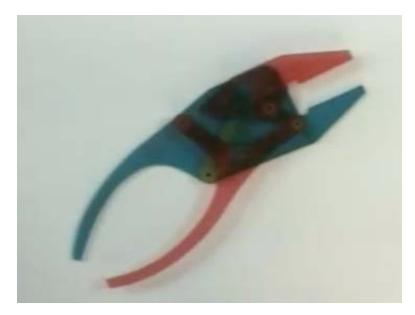
However, we can design parallel job players by using a suitable mechanism. Using this mechanism, as we see the upper jaw is moving parallel to the lower jaw and consequently it will provide a very good grip on a flat object. So in such mechanisms, the generation of these specific motion characteristics is a primary interest rather than the forces on top invert.
