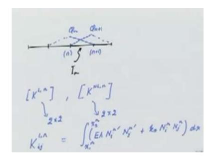
The question is how do we do it at the element level again we have let us say a mesh of some elements. Let me pick a generic element I,  $I_n$  in this element, let's say I have these basics functions which are non-zero. I am taking a linear approximation to bring the point out. I will be corresponding to the node n and n plus one phi<sub>n</sub> phi<sub>n+1</sub>.
