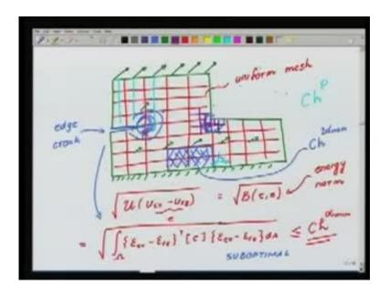
So, with this approach, with a graded refinement, we can capture singular behavior of the solution and then, just like I talked about earlier, in the crack tape, in the vicinity of the crack tape, there are methods by which I can abstract, what is known as the stress intensity factor, the k, that we can abstract with much better accuracy if I used this kind of a graded machine.
