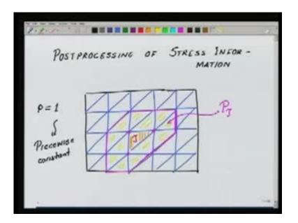
Here, we are going to continue a discussion further with a planer elasticity problem. And, as we had done in the one-dimensional problem of the bar and the beam, we will continue here with the desire to obtain a better state of stress from the finite element data that has been obtained; that is, we are interested in the post processing of the stress information.
