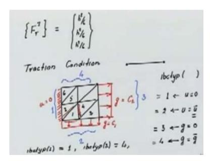
I find that the first edge of the element lies on the boundary edge two. The boundary edge two has an ibc type which is four and now I can go ahead and do the integral of the given g on this edge against the shape functions which are non-zero on this edge.
