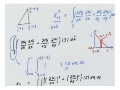
The Jacobian is also constant so our integral gives us, let us say I want to find  $k_{11}$ , will be equal to integral over the psi integral over the eta of del N<sub>1</sub> del x whole squared plus del N<sub>1</sub> del y whole squared into Jacobian into d eta d psi. For us this del N<sub>1</sub> del x whole squared will be equal to (del N<sub>1</sub> del x is equal to minus 1 by h, del N<sub>1</sub> del y = 0), let us put that and Jacobian is equal to h squared.
