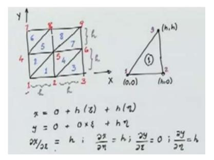
For this domain, I would like to do the element stiffness matrix calculations using the linear approximation over the domain. Let us go through the steps that we have done earlier. Let's take element 1 as an example. Element 1 is this. If I look at the coordinates of element 1, say, the coordinate system that I have employed is like this: this is the origin o, this is the x-axis and this is the y-axis. The coordinates of the N nodes of the
