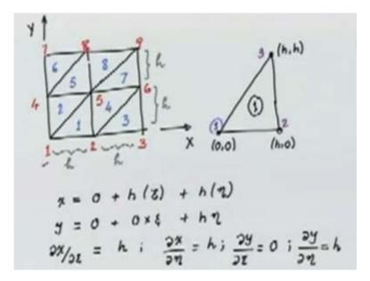
If I do that numbering, then I am actually following the numbering which I had done for element 1. If I turn the element 1 around, that is, rotate it around, I will get exactly the same local numbering as I had done for element 2.
