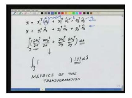
Geometry mapping becomes x is equal to  $x_1$  of tau into  $N_1$  hat plus  $x_2$  of tau into  $N_2$  hat plus  $x_3$  of tau into  $N_3$  hat and y becomes  $y_1$  of tau into  $N_1$  hat plus  $y_2$  of tau into  $N_2$  hat plus  $y_3$  of tau into  $N_3$  hat. This is how I can give the x and y at any point psi and eta in the master element, the corresponding value of x and y.
