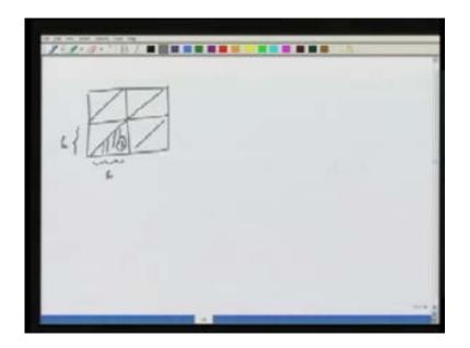
Given these elements of size h, I would like to construct, let us say, for the first element in my domain, the entries of the stiffness matrix using linear approximation.
