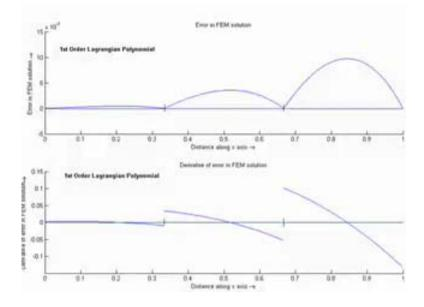
If I have P is equal to 1 let us look at the next figure. From the next figure, we see that the error at the corner node is 0 and because it is the same problem that we have taken the exact solution of x power 4 defines that the error at the node value is 0.
