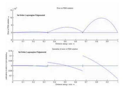
We see that at the end points of the element, the derivative of the finite element solution is very far from the exact form. If we look at the error plot, this error is quite high at the nodes of the elements. This is very important feature of the finite element solution. In fact this is the
