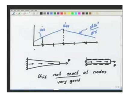
We find that at the mid point of the element the derivative is very good. We can pass a straight line between the values of the finite element derivative of the finite element solution so that straight line this is  $u_{FE}$  prime at this point  $u_{FE}$  prime at this point.
