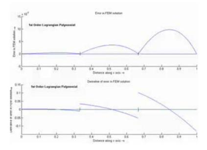
In the second part of the figure we will note that the derivative of the error vanishes at the midpoint of the element.
