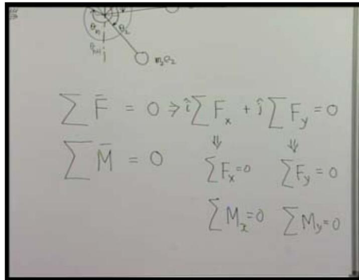
The image shows a whiteboard with handwritten mathematical equations. At the top, there is a small diagram of a mass  $m_2$  at a distance  $r_2$  from a center, with forces  $F_x$  and  $F_y$  acting on it. Below the diagram, the following equations are written:
