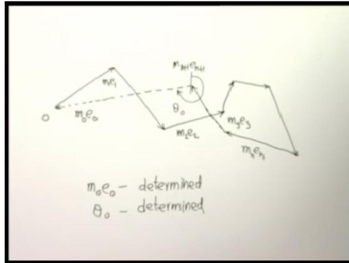
The force vector diagram will be again, will start from 0. This is  $m_1e_1$ ,  $m_2e_2$  will be in this direction,  $m_3e_3$  will be in this direction and then we have two more as placed here. This is  $m_n e_n$  and even this one is known to close the polygon, your  $m_0e_0$  which is the only other one force left must be this. Again, we find out its angular position  $\theta_{a_0}$  and its magnitude  $m_0e_0$ . Thus,  $m_0e_0$  is determined and of course  $\theta_{a_0}$ .
