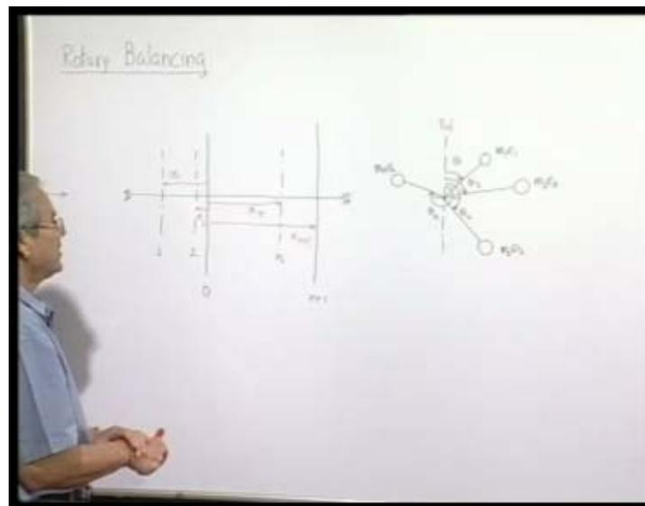
Today, we will take up analysis of such rotating systems and find out the masses which are needed to balance such a rotating system at the design stage. So, let us take a rotating shaft that carries  $n$  number of unbalanced masses; let the plane of this unbalances be 1, 2 and so on up to  $n$ . **When we view from this side the angular position of this unbalances are as shown in this slide (Refer Slide Time: 02:00).**
