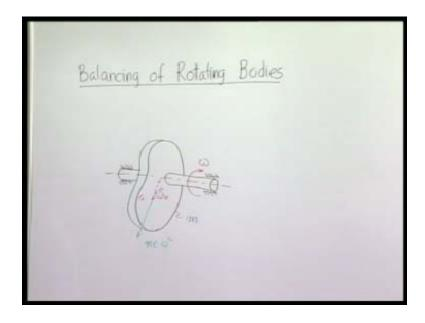
Let us take up a simple case. When an object is mounted on a shaft which is rotating, let us see what will be unbalanced force experienced by the bearing or the support. Now, we know that there can be two situations. The object itself may be of irregular shape by virtue of which the center of mass is away from the axis of rotation, and let the eccentricity of the center of mass be denoted by e, and let the mass of the whole object which is rotating be m.
