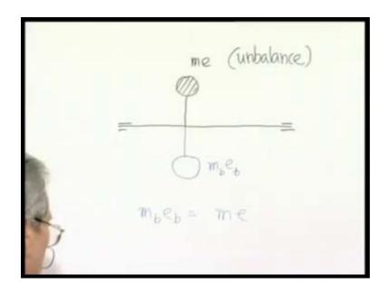
We have a simplified way of representing a dynamic body, rotating dynamic body. If this be the support axis, then let this be the eccentric mass and now as we find that it is the product of the mass and eccentricity which determines the force, this (()) is omega. We will always represent the unbalanced as a product of mass of the object and the eccentricity of its c G from the axis of rotation.
