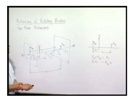
Now, any force here can be represented by two forces; that means, suppose if I have a force acting here F, I can always represent it by two forces at any two points by F 1 A and F 1 B, so that these two forces' resultant is F 1. So, I can replace the force by this. So therefore, what I can do?
