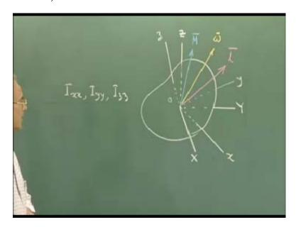
So that the products of inertia terms are zero, only the moments of terms of inertia are present. Then the moments of inertia of this in the various directions are  $I_{xx}$ ,  $I_{yy}$  and  $I_{zz}$ .
