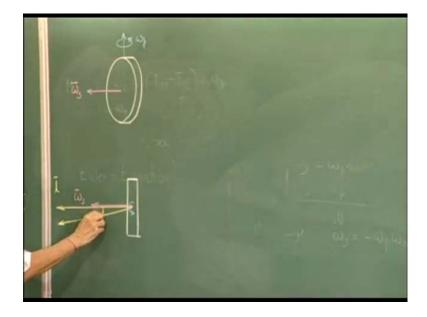
I am giving a rotation about this axis, so that means I am giving a rotation about this with a velocity  $omega_p$ . In time delta t the whole thing will come somewhere here, this is the new angular momentum vector. How much will the angular velocity be? It is  $omega_p$  into the time, which is delta t. This is nothing but  $omega_p$  into delta t. This angle is the change in angular momentum because, original angular momentum plus the change makes the new
