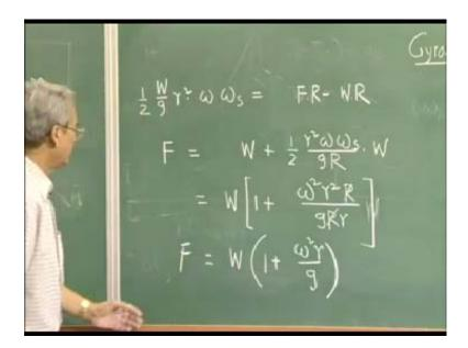
May be a 10 ton roller can produce a 15 ton crushing force. This is an advantage we get, so this kind of an effect that brings the forces or bearing reactions or moments, which all get generated because of the Gyroscopic action, must be taken into account. Whenever a rotating body changes its axis of rotation, there the gyroscopic action will come into action. There are many examples where you will find that the there are like a fly wheel of a car it is quite
