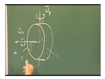
Now we should remember, since the rigid body is rotating continuously about the x-axis, the location of y and z-axis continuously changes within the space. What we can say, that these are not the instantaneous position of the x, y and z, rather this x, y and z will be the instantaneous axis, which is rigidly attached to the body and rotating along with it.
