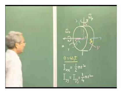
If we now apply this to a simple problem, which we encounter in engineering quite often where a disk that is rotating with an angular velocity omega<sub>s</sub> about its central axis, which has a mass m and radius r. If this body is given a rotation about an axis which is perpendicular to this angular spin, angular velocity omega<sub>s</sub>, when this is 90 degrees, for this motion, if this is the motion, then what are the externally applied moments on this?
