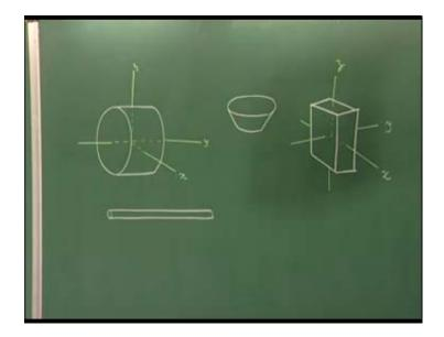
The difference between this and this is that here only y direction is fixed, x and z can be any two mutually perpendicular directions, where both x and z are at right angles to y. In this case that is not so, they are the direction of x y z are all uniquely determined. Similarly, we will find that in this case again it is an axis-symmetry body. So, this will be one principal axis and then any two mutually perpendicular lines because of this circular symmetry can be principal axis.
