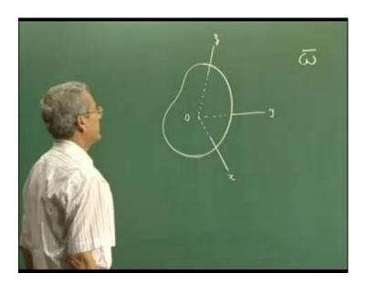
If this be the rigid body under consideration, its translational motion can be considered to be a particle type of motion, where the whole mass of the rigid body may be considered to be concentrated at this center of mass. The angular motion, about the center of mass or any other fixed point o can be represented by an instantaneous angular rotation about an
