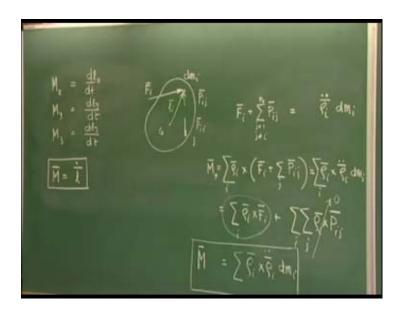
This is the center of mass G; say the ith particle with a mass  $dm_i$ . The external force which is acting on this ith particle is  $F_i$  and this particle is subjected to interactive force with other particles apart from this external force.
