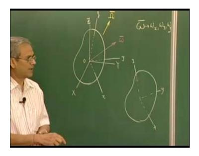
This rigid body is now, along this direction x, along this direction y and along this direction z. If I measure or define its moment of inertia about the x axis is  $I_{xx}$ , the moment of inertia about the rotation axis y is  $I_{yy}$  and moment of inertia for the rotation about axis z is  $I_{zz}$ . These were familiar terms. We have seen the concept of moment of inertia even in planar motion of rigid bodies in our dynamical courses.
