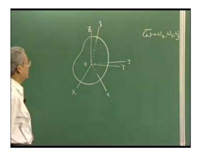
We should also remember that there is another set of coordinates - capital X, capital Y, capital Z. Without losing much generality in the results we can make the two origins coincide at o. This smaller x y z system has an instantaneous or an angular velocity omega with respect to the fixed frame of reference.
