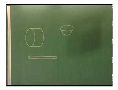
In most cases, these are the kind of component shapes we will be dealing with and for such cases it is easy to determine the principal axis by observation. If the body is symmetric, then all axis of symmetry will be principal axis. So, in the case of that roller, for example, Y axis of symmetry is very obviously this one. So, this will be one principal axis (Refer Slide Time: 10:33).
