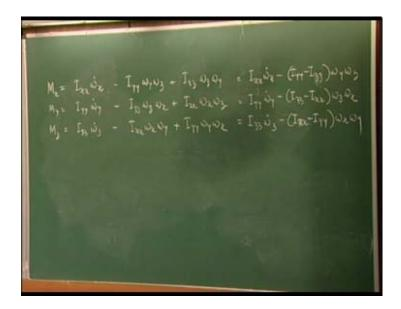
As it was first derived by Euler and this is the form of equation, though it is not perfectly general. The perfectly general form will be like that where the small x y z system is not rigidly attached to the body. We will do some such examples in the next lecture, if we get time, but this will be the governing equations for all the rigid body motions in three dimensions; we will be doing and we will be applying to machines.
