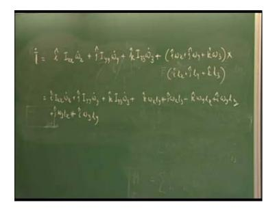
Now, remember that this l, rate of change of angular momentum is nothing but the externally applied moment. So,  $M_x$  will be the x component of this. That means the terms if we take i hat as common, the term with which i is associated and that will be  $I_{xx}$  omega x dot plus i omega<sub>y</sub>  $l_z$ . Now,  $l_z$  is nothing but  $I_{zz}$  omega<sub>z</sub> and the other term is this minus omega<sub>z</sub> I  $l_y$  is  $I_{yy}$  omega<sub>y</sub>.
