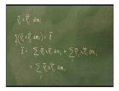
Let me see; to show this, we will start with rho i dot is the velocity of the particle, when multiplied by dm<sub>i</sub> we get the linear momentum of the particle. So, rho i cross the linear momentum is by definition the angular momentum. If you sum it up for all the particles, we get the angular momentum vector for the rigid body. This is the expression for angular momentum of the rigid body about point g from where rho i is being measured.
