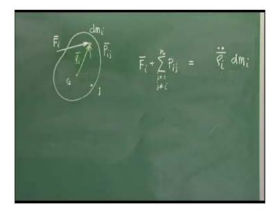
Therefore, you will find that if the position vector of this be rho i, then the moment or rather the total force, first of all, is  $F_i$  plus  $P_{ij}$  j from 1 to n except j is not equal to i. So, that is the total force acting on the particle. If this is a fixed point, we can show that this will be nothing but  $dm_i$  is the mass and  $P_{ij}$  is the acceleration of the particle.
