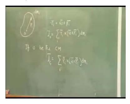
Let us now investigate little bit about the inertial property of a rigid body in space motion. If we take the angular momentum of a rigid body, if the particles be infinitesimally small and the number become infinitesimally large, then we know that the summation can be represented or replaced by integration over the whole body (Refer slide time: 35:58). Now we would like to have a more clear definition or rather in more concrete terms this quantity.
