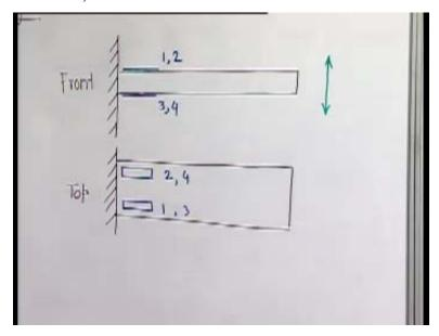
These are the two views: one top view, one front view. The top view and the front view at the same ((calculated beam)). Now when it vibrates; vibrating means it bends, what happens? It stretches like this when it goes down, so the outer surface will be extended and the lower surface will be compressed.
