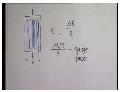
Now, I think again, what are strain gauges? It is known, but even then I will just give a very quick overview. The strain gauge is a very small, maybe one centimeter by fraction of a centimeter long, a (( )) kind of thing in which it is embedded to a very thin wire. Now to have a large length of the wire, we have to loop it like this, so the total length of the wire is very large and the resistance is measurable, but the overall dimension of this is small.
