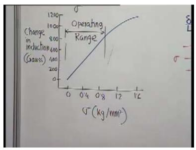
This is the change in induction in Gauss; it will be 0,200,400 like this. This is the realistic values for a particular case, so you can see that the operating range could be very easily found (Refer Slide Time: 24:09). This of course, you can really understand that if you have to attach it to the plane vibrating body, this becomes contact type.
