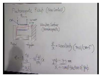
First, let us take a non contact type pickup based on electromagnetic induction. The basic scheme is shown. This is the coil; it is wound about one leg of this permanent magnet; this is the vibrating surface; it as to be ferromagnetic; this is the gap maintained and this is vibrating.
