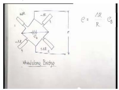
Now resistances or these strain gauges, I am representing like this, not that they are physically kept like this, but thus electrical circuit point of view am just keeping like this. If it is 1,2,3,4 and the circuit will have this kind of arrangement that means, which is called Wheatstone bridge. On principle, we could sense the resistance variation of only one strain gauge, but the sensitivity will be low.
