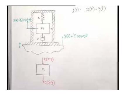
So, this is the basic scheme of the pickup, it is connected to a machine body or system body which is vibrating like this (Refer Slide Time: 30:20) and we call this vibration as a function of time. Then, we know that from equilibrium position the vibration of the mass we can describe by x, which is a function of time given by X. Now in such a situation
