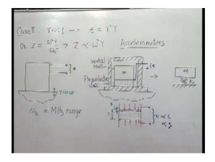
Now, both these conditions are very nicely satisfied by one type of pick up where this is the inertial mass mounted on a thin disk of a special kind of material which we call piezoelectric material.
