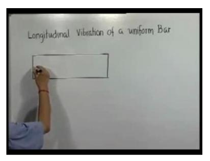
So, first case is the longitudinal vibration of a uniform prismatic bar. This is our uniform prismatic bar. Whatever may be the cross-section it is uniform and we now fix of a coordinate system attached to the body with one end as the origin. Then, we consider the technique of solving this kind of problems to be used is to identify an element at any general location x and find out what will be the dynamics of the element which is valid at
