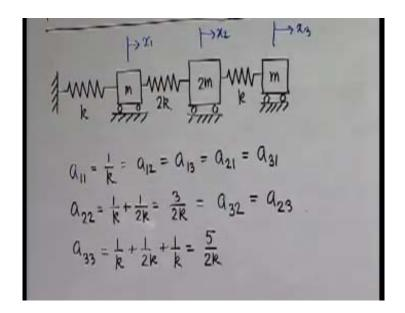
Let us consider the three degree freedom system. This is simple three degree freedom system and our objective is to find out the natural frequencies and the natural mode. First, we have to determine the D matrix, m matrix is quite straight forward but D matrix we have to find out the flexibility matrix. Let us see, what is  $a_{11}$  that is, if you apply a unit load at station one what is the deflection of station one? Obviously, it is only the space of string and that is nothing but 1 by k.
