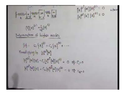
If we could somehow make  $C_1$  zero then our assumed shape would have started from here and if we repeatedly multiply or pre-multiply this by D then the whole thing will convert to the second mode and we will get the second natural frequency. Similarly, if we could make both  $C_1$  and  $C_2$  zero by some means then the whole thing the next term it
