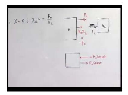
Now, what will be happening if this is the auxiliary system and this is the main system, then the force which is acting here, it will be simply  $k_a$  into  $X_a$ . Of course, there is another force here, which is  $F_0$ . Now, how much is this under this tuned condition? It is minus  $F_0$  plus every instant of course when you multiply by cosine omega t in both the places, what happens?
