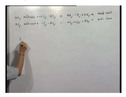
Substituting in these equations we get (Refer Slide Time: 40:00), c omega rho is nothing but velocity of this point. If we multiply by sine theta, what happens, it is the x component of velocity of o prime point. It is nothing but c into  $x_{oprime}$  dot.
