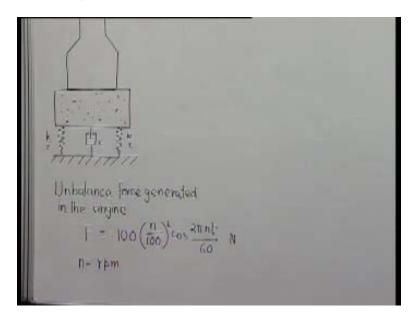
This is a vertical engine, is supported on a concrete block. This concrete block again in turn is resting on a system of springs, with total resultant stiffness of k and system of dashpot, total resultant damping coefficient c.
