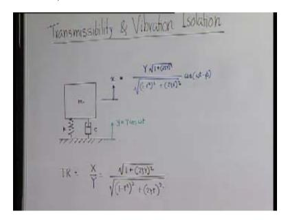
The main objective of this study will be, how to decide the parameters like stiffness and dashpot, viscous dashpot, damping coefficient in a manner, so that the system can be isolated from the environment.
