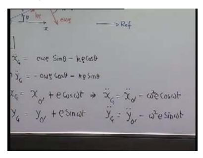
We can also represent  $x_G$  and  $y_G$ . This  $x_G$  is equal to  $x_{oprime}$  plus e cosine omega t and  $y_G$   $y_{oprime}$  plus e. This will give me  $x_G$  two dot is equal to  $x_{oprime}$  two dot minus omega square cosine omega t and  $y_G$  two dot equal to  $y_{oprime}$  two dot minus omega square e sine into omega t.
