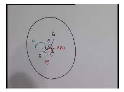
Therefore, if distance is e eccentricity which is inherently present, because of wrong manufacture or fabrication and this distance is rho. Rho represents the deflection of the shaft due to the unbalanced force produced. Now, what are the forces acting? External forces acting on the disc let us see that. The shaft has been bent, when you bend a shaft,
