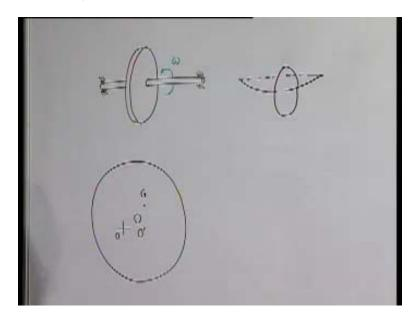
One, very common problem faced by mechanical engineering is the shafts carrying discs. A shaft like this is rotating with a speed omega. Now, whether there is any potential problem, the dynamics of rotating bodies itself is a subject. We will not be able to discuss it there, but the simplest possible case we would like to take up, because it has lot of similarities in all kinds of analysis we have been doing.
