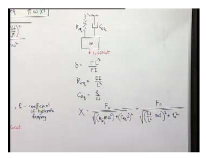
So its equivalent rigidity is going to be simply then EI by L cube. Similarly c equivalent is going to be  $E_d$ , which is c equivalent is going to be h by omega. So when it is subjected to a harmonic force (Refer Slide Time: 27:28), the displacement which we will get x will
