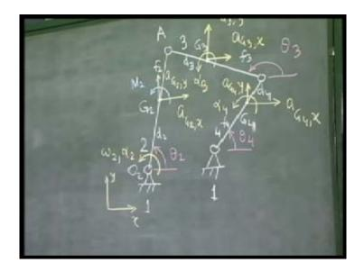
Lets us explain the procedure with the help of an example of the four link mechanism. Let our mechanism be this; this is the moving link 2, this is the moving link 3, this is the moving link 4 and the fixed link we always call as 1, as you know.
