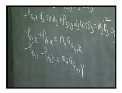
I have already mentioned that since the kinematics is completely solved we all know the acceleration components and the angular accelerations. For the last link, exactly in the same procedure, we will get total equation in the x direction as minus  $P_{43,x}$  plus  $P_{14,x}$  this must be equal to  $m_4$   $a_{G4,x}$ ; in the y direction, we will have minus  $P_{43,y}$  plus  $P_{14,y}$  and this is equal to  $m_4$   $a_{G4,y}$ .
