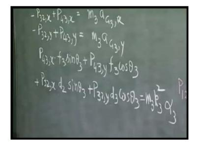
Therefore, the momentum is this; it will be equal to  $F_3$  sine theta<sub>3</sub>; this is the moment of this about this.  $P_{43,y}$  will also apply a moment about this, with this as the momentum. (Refer Slide Time: 21:21) This also will produce clockwise moment  $P_{32,x}$  d<sub>2</sub>; momentum
