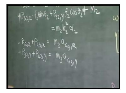
Exactly in the same way, when you go to other links, we can write down similar equations like minus  $P_{32,x}$  plus  $P_{43,x}$  which is equal to  $m_3$   $a_{G3,x}$ , minus  $P_{32,y}$  plus  $P_{43,y}$ , which is equal to  $m_3$   $a_{G3,y}$ . Then by taking moment it will be,  $P_{43,x}$ ; this is  $F_3$ ; this length is  $d_3$  and this angle is theta<sub>3</sub>. (Refer Slide Time: 20:40)
