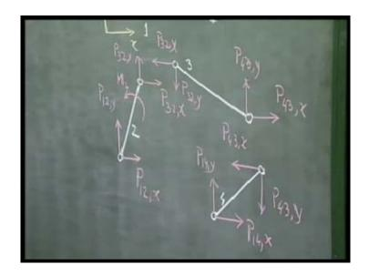
Next, let us draw an excluded view of link-mechanism. The joint forces, say this particular joint which connects link 2 with link 1, the components of forces be  $P_{12,x}$  and  $P_{12,y}$ , it means it is the joint force from link 1 on link 2, in the x ((component)) direction and y direction.
