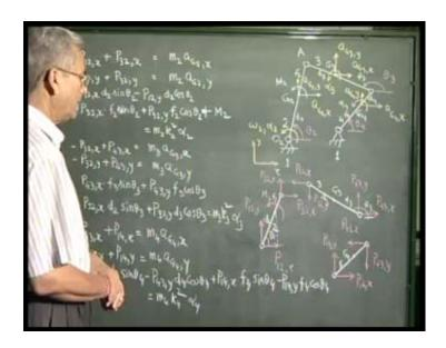
In the graphical procedure, it becomes extremely difficult to repeat it hundreds of times for getting analysis of one complete cycle. Once the forces are known, then of course a designer can design the bearings and other joints suitably so that such forces can be sustained. It is also possible, but we are not going to do here, once you have force on each link, it is also possible to find out these traces which they are subjected too and their design can be taken care off.
