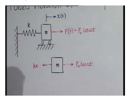
At any instant of time, the forces acting on this will be kx. So, total acceleration in this direction x two dot multiplied by m has to be total force in that direction.
