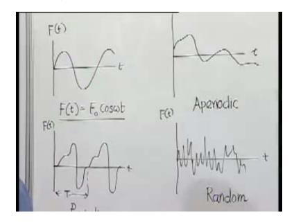
Excitation of a system can be of various types. First of all, we will classify the situations according to the nature of the forcing function or the disturbance. If the forcing is purely a harmonic function of time, say if we call this is the force, so this is called harmonic excitation (Refer Slide Time: 03:39) because the excitation, the function of time is a harmonic function of time.
