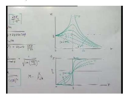
The characteristic looks like this, if we plot it, magnification factor is defined the same way here, X by  $F_0$  by k. As we can see, when r is tending to 0 when it is simply, this is 1, this is 0, so it will be 1. This way now of course, we have a parameter like zeta, for different values of zeta, we will get different result. So, zeta is increasing in result and this is zeta equal to 0.
