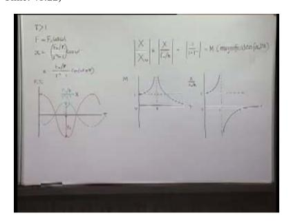
This case x will be as shown in the above slide. I want to keep this always a positive quantity, so we can write this as r square minus 1 and take minus sign here. We can write this as  $F_0$  by k divided by r square minus 1 into cos omega t plus pi. Therefore, what will happen now is that the forcing function and the displacement or response will be just out of phase.
