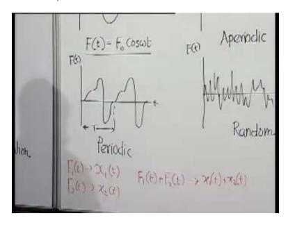
As we are dealing with only linear systems, if a particular forcing function gives a response  $x_1$  and another forcing function  $F_2$  gives solution  $x_2$ , then when both are combined they will give the response  $x_1$  t plus  $x_2$  t. This is a very important result, but valid only for linear systems.
