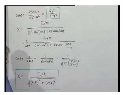
The first equation will tell us X is equal to (Refer Slide Time 54: 10). So, we take X common and divide  $F_0$  by m by the coefficient of X. So, if we take cosine phi common outside, we get  $F_0$  by m by cosine phi, if we take 1 by cosine phi, then it is omega square minus omega<sub>n</sub> squared plus 2 zeta omega<sub>n</sub> into tan phi. Tan phi is already determined, is 2zeta r by 1 minus r squared.
