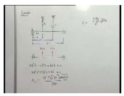
The system is like this, a mass less rigid rod is hinged at o is approximately horizontal position, and carries a mass concentrated mass m at the distance from the hinge. A spring is attached of thickness k, at a distance b from the hinge. A viscous dashpot of damping
