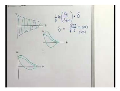
The viscously damped single degree freedom system, and their vibration characteristics, I think we have to take up the case of the system, where we have solid friction. That means coulomb damping, and the next lecture we will take up the single degree freedom systems with coulomb damping. It is the vibration.
