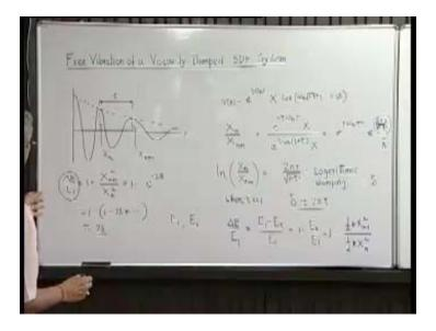
Now this is a measure of the intensity of the damping that means how fast the amplitude is reducing. Higher the value of this ratio of the two successive amplitudes, larger is the damping and when you take the natural logarithmic of the ratio of the two successive, you
