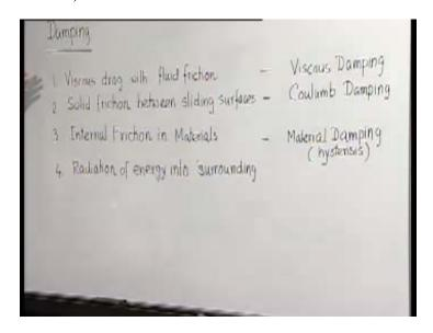
Sometimes we may find say for example, the pin of the pendulum in its hinge. If it is not properly lubricated, that may give rise to a solid friction between the housing or the journal of the bearing and the bearing itself of the spline. Similarly, there can be other situations where vibration or vibrating system may involve two solid objects rubbing against each other and that will give rise to Coulomb damping.
