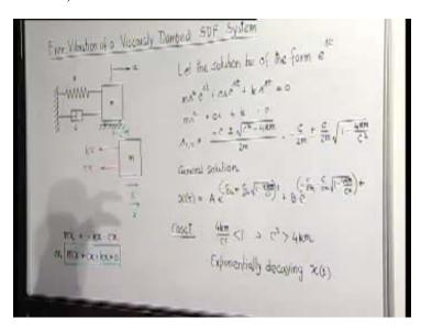
The natural length position, because if the spring is stretched or compressed, it will again slowly either go out or come back, so that this mass can come to that position when no force is acting on it. That means when it is stationary, so no viscous damping force and this spring is at natural length to known compression or tension force in that. When we displace it, mass is here, there will be two forces that will be acting. As we know, at any instant its position is
