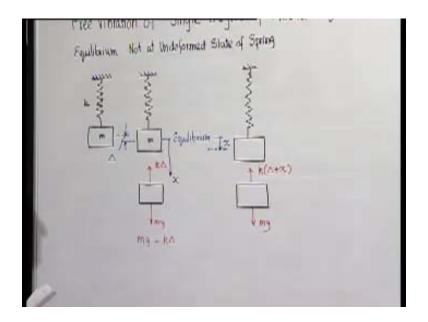
Now, what is the equilibrium situation? What does it signify? The total vertical force on this mass, one is the weight mg and other the spring force which is k into deformation of the spring delta. Since it is equilibrium, mg must be equal to k delta. We measure the displacement always from the equilibrium position. Now finally, we give some further deformation or displacement to the mass from its equilibrium.
