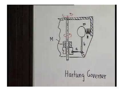
Today, we will discuss two important such governor mechanisms, which fall in the class Spring Controlled Centrifugal Governors. This class of governors also operates on the basis of the reflecting force, which is nothing but the centrifugal force, which are controlled predominantly by springs.
