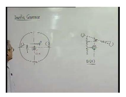
So, I just give one quick example of inertia governor (Refer Slide Time: 49:58). This type of governor is called Inertia governor or flywheel type governor. I am not going into the detailed analysis; I will only indicate the basic features of such system. This is like a disk mounted on the top and is rotating in this direction at speed omega. Now, there is a lever hinged at location say, let us call it A.
