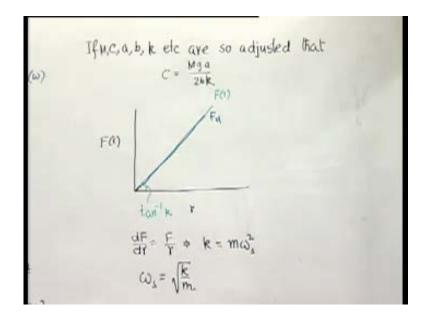
If that is done, if M, c, a, b, k etc are so adjusted that c is equal to Mga by 2bk; if we do that then what happens? then this becomes 0, the control force diagram will now look like this (Refer Slide Time: 15:32). What does it indicate? The system can have equilibrium condition only if the deflecting force also coincides with that. This indicates that we have already seen this kind of situation which is called isochronous situation or the governor is isochronous at the speed.
