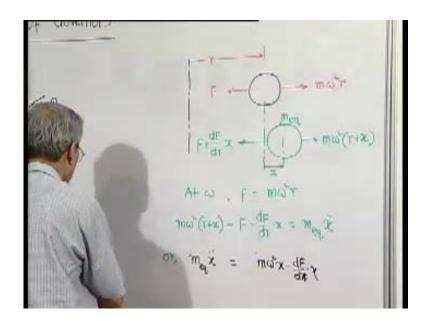
Now, how to find out the natural frequency of the governor, its operation? We can do an approximation analysis like this. This is the spherical ball and the forces are as we have seen that in the equilibrium position; this is F and this is m omega square r; this is r. Now, due to some disturbance it has shifted here (Refer Slide Time: 43:43).
