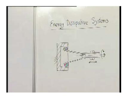
This is rotating the shaft coming from the system and there are two leaves spring very thin spring, at the end there are two brake shoes kind of thing. The length of this can be adjusted so that sometimes it go nearer to this up and sometimes it can be down.
