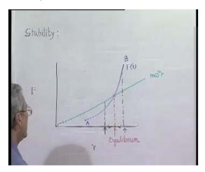
Next important point, we have to keep in mind is stability of operation. What is stability? Stability has it is defined in many other cases. There also stability is defined by the situation what happened if the system is displays from its equilibrium; it displays the configuration little bit from its equilibrium running condition. If it comes back to the original equilibrium position it means governor running stable back.
