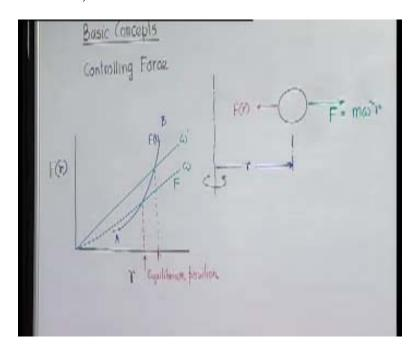
This control force is the function of radius, so you can say it can be something like this; in general, it will be a curve something like this (Refer Slide Time: 34:33). When it is rotating at some speed this force will generate centrifugal force, which is nothing but m omega square r, where m is the mass of the sphere. If you plot this for a particular speed, omega is a straight line, this is F and this is Fr control force.
