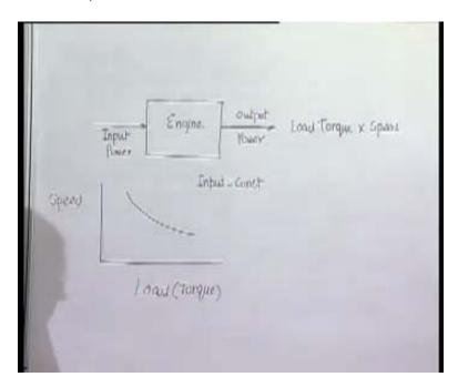
Now, let us see how or what are the parameters from which speed of running an engine - let us take the example of an engine, will depend. In a schematic form of an engine or general mechanical system, there is input power in the form of heat or whatever it may be in case of engine and we get output power. For example, engine is generating current or pumping water or running a machine tool whatever it may be and this output power – it means what? Load torque multiplied by operational speed.
