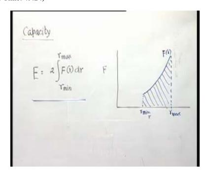
The other term we should be finalizing with other characteristic will be capacity. I already mention that the governor has to do some physical work also by operating the whole ball control mechanism. So, it is important to have enough capacity; what capability of the governor, this is defined as which is nothing but work done, this is the control force curve between the minimum and maximum operating radius.
