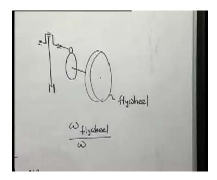
Now, this is solved in this manner. If you have this crankshaft and this is a punch rather than directly attaching the flywheel with this, we use gearing system and we attached the
