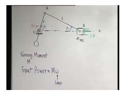
If we consider a case, where the input speed or the running speed omega to be approximately constant, then what really tells about the fluctuation of input power is also same as the fluctuation of turning moment which is M, because input power is nothing but M into omega. So, when we take this as constant then fluctuation of M or turning moment is the critical thing and that is what we have to find out. To do that we again
