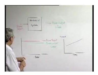
What is going to happen? The speed at which this mechanical system is operating will gradually change and in this case, we will find that with time the speed of the machine will gradually increase, because with time more and more energy is going to remain into the system and resulting in gradual increase in the kinetic energy; that is the speed of this. The reverse situation is there, where it can be less.
