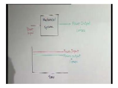
If we take a mechanical system, then its condition can be generally specified by two things. How much power input is there and how much power output plus losses are there. So, what is happening in a mechanical system? Irrespective of the nature of the system,
