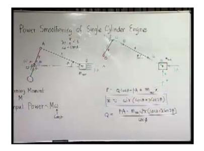
Our objective is to find out the turning moment M acting on the crank pin. Let us first find out Q. Now, the resultant force on this will be in this direction which is F; it has to be in this direction because the piston can accelerate only along x direction. We know F is equal to - now this angle is phi - Q cosine phi minus p A and that must be equal to the  $m_{reciprocating}$  into the acceleration in that direction x two dots.
