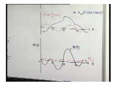
That means, total area bounded by the black curve and the red line above and below will be same. It is quite clear that in such a situation a substantial amount of fluctuation of energy, here the load is more than the input up to this; then slightly input is more up to this; again load is more than input; then here input is more than the load and so on (Refer Slide Time: 54:25). Therefore, there will be substantial amount of fluctuation of speed and such.
