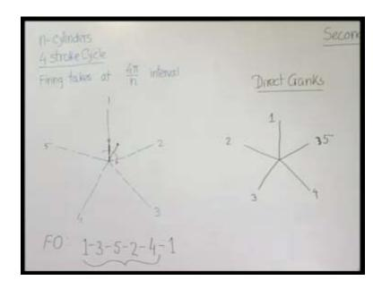
Thus the only remaining primary unbalance force is 5 by 2  $m_{reciprocating}$  omega square by omega square r and that can be balanced by placing counter weight just opposite to the actual crank; this is okay.
