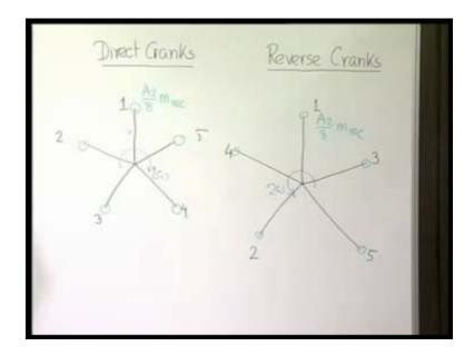
If we place then how much mass we have to place?  $A_2$  by 8; this is r; same here; same here; same here; same here (Refer Slide Time: 42:45). This is direct crank; they all are rotating in this direction at speed omega. The centrifugal force produced by the eccentric masses placed at the crankpin of the direct crank of the direct secondary crank; you can see they are balancing among themselves.
