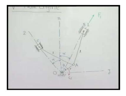
It should also be remembered, though we are referring to these systems of engines, there can also be compressors and other types of machines. In V Twin Engine, two identical cylinders rotates a common crank, if both of the connecting rod are identical with length l, then crank is called as common crank.
