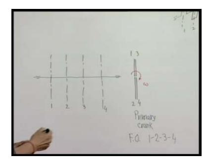
Then, first number 1 which is here, then next 2 comes up 180 degree rotation of the crankshaft; then number 2 expires; then number 3 comes up after total of 2pi that means after 2 it will be again another pi; when 3 comes up, then that fires and then finally, another 180 rotation and crank 4 cylinder number 4pi. So, this will be the isometric view of the common crankshaft.
