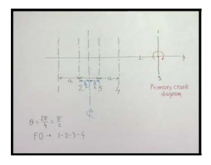
Of course, the primary crank is rotating in this direction. One should never forget to indicate the direction of rotation; otherwise, this firing order has got no meaning. Let us see what happens, if we consider that the reciprocating mass of the cylinder and the portion mass of connecting rod at the cylinder, they are placed here at the tip of the cranks.
