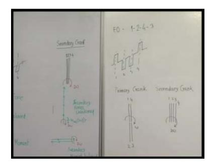
You will see; what actually you want to tell now, which is very important that just by changing the firing order it is possible to include balancing situation. Suppose, the same engine we take the firing order as 1- 2- 4- 3 that means first cylinder fires, then second cylinder fires, then fourth cylinder fires and finally third cylinder fires. This will be the isometric view of the common crankshaft 1 2 3 4 and crank diagram will be as shown in slide for primary crank.
