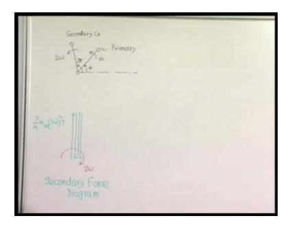
Here, you can see the secondary force diagram is also closed polygon because we have come back to this same point where you start it and from this we find secondary force is balanced.
