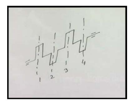
In case of 4 cylinders 4 stroke cycle engine, the angle between the consecutive firing cranks will be 4pi by 4 that is equal to pi and say, this is the system. The primary crank diagram will look like this, suppose we start with firing of 1 and if the firing order we keep as 1-2-3-4.
