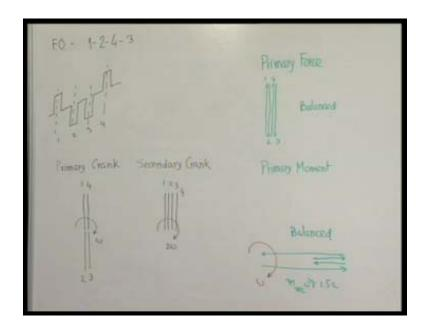
Whatever the secondary, when you draw the secondary crank 2 into 0; that is for cylinder number 1 or crank number 1 it will be 0. Then 2 it is at angle 180 degrees or pi; so, two of that will be 180 degrees it will be like this. Then, 3 is also again 0 so two of 0, 2 into 0 will be again 0 and 4 is again 90, 180 degrees two of that will be again.
