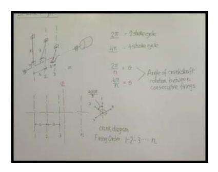
If there are two equal and opposite forces, passing or acting along two different lines of action, then they produce a couple and that can produce unbalanced forces on the supporting bearings. Same thing here, because we have seen that the unbalanced primary force of each one can be represented by placing a mass of the cylinder here and assuming that only the component along this cylinder centerline that is only existing, rest is not existing.
