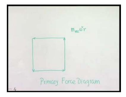
If those centrifugal forces they themselves got balanced then obviously, there components along any direction will be also balanced. For cylinder number 2, the unbalanced force produced is this of same magnitude at 90 degrees. The centrifugal force produced by the third cylinder with that mass here will be this and by fourth cylinder will be this. Therefore, we call it primary force diagram.
