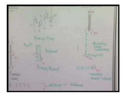
Primary forces or secondary forces are unbalanced; now secondary moments we will find will be balance because this will produce four moments in this direction. Then this will produce again a moment in this direction, then this will produce again a moment in the opposite direction and this center four will produce a moment in this direction and whole thing is rotating; both these also rotating and it is started here. So, you come back therefore resultant is 0.
