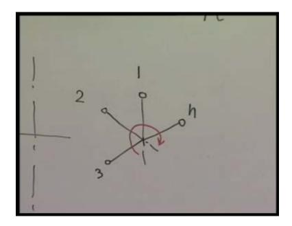
We can have a crank diagram which we call as for cylinder number 1, cylinder number 2 crank, cylinder number 3 crank and so on; so, this is cylinder number n crank. We have to also indicate always in a crank diagram the direction of rotation we know say, the direction of rotation is this. Therefore, we can see from this crank diagram, we can also find out the firing order.
