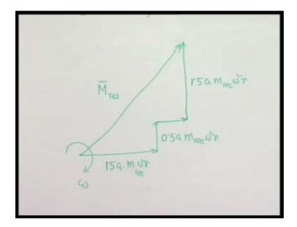
Since, all forces are in vertical direction, in reality. So, the real moment will be always in the horizontal direction. The component, along this is the real moment or actual moment. So, when this is at this position making 90 degree with this direction, then moment is actually instantaneously it is 0. When moment is aligned with this vector, then the total moment it is exactly its magnitude is same as m reciprocating the maximum ((null)).
