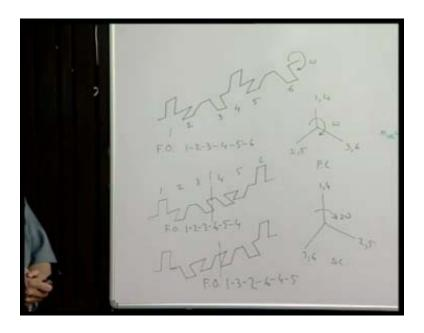
You can see that replace mass at the crank pins; primary force will all balanced because there are symmetrically placed, secondary force will all balanced as there also symmetrically placed, but primary moments and secondary moments not be balanced. To achieve, both primary and secondary force balance, and to achieve primary and secondary moment balance that is complete balance up to secondary, we have to take crankshaft which are symmetrical like this or its 1- 2- 3- 4- 5- 6.
