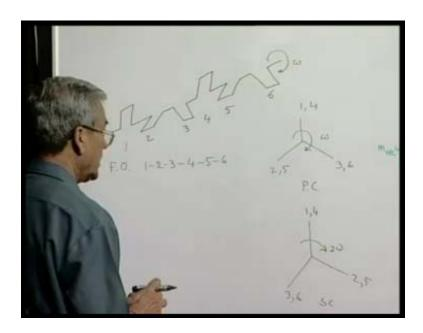
This is the primary crank, so 1 2 3 4 5 6 this is primary crank; secondary crank, one will be same because 0 into 0 is 0, 2 the angle is 240 degree, double of that is 480 that means 360 plus 120, 2 will be here, then 3 is 120 double of that is 240, it will go it in the direction, 3 will be here, 4 will be again here, then 5 will be here and 6 will be here, this will be secondary.
