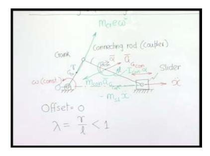
This single slider machines are very common in large types of machines, then compressors, engines, they all employ this mechanism. So, I think it will be appropriate to take up this particular case and investigate it unbalance and also look into the ways and means of balancing the unbalance present.
