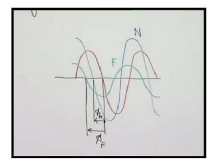
This oscilloscope signals tells that this is the phase lead of the near-end response or near-end sine wave, which you get and this is the far-end. The near-end response we get as  $N_1$  vector and obviously, the reference is here. Reference vector is nothing but the sine-wave generator, so this will be phi subscript N. Similarly, at the far-end again the reference will be same, this will be phi subscript F and the vector representing the vibration of the far-end is  $F_1$ .
