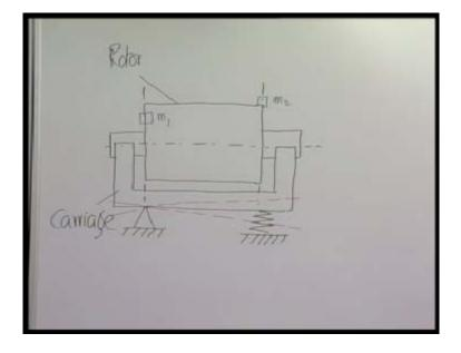
If you have a rotor like this, rotor is placed on a carriage, the carriage has two half bearings. Now, we take a pivot to support one end of this carriage and the other end is supported on a spring. Now once this rotor starts rotating, then the centrifugal force or unbalanced inertia forces will start appearing depending on the speed of the rotor.
