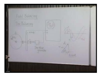
This will be pickup A and this will be pickup B. We will draw it in a slightly bigger. This is the sine-wave generator.
