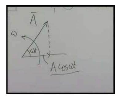
A rotating vector can represent any harmonic function of time when we consider only the component of that rotating vector as the real quantity. If this is a vector A rotating with a speed omega, then at any instant this is omega t and its magnitude is simply A cosine omega t, a harmonic function of time. We will just represent the vibration when it is rotated at speed omega by  $A_1$ .  $A_1$  magnitude is this and its location from this reference is this, where this angle is phi subscript 1.
