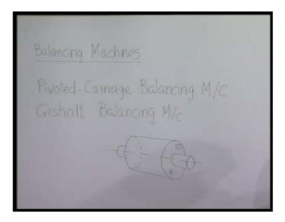
It is easier to add a mass here or the same result can be achieved if some mass is cooked out or removed from a diametrically opposite position. The effect will be same as adding a mass here. Therefore, these faces of the rotors may be chosen as the balancing planes. Anyhow, this is just one particular case, so it will depend on the situation.
