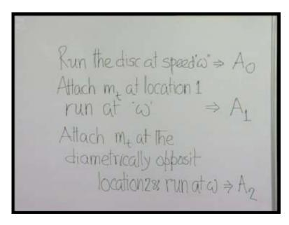
We take the disc, rotate it at a suitable rpm or suitable speed omega and measure the vibration amplitude A. We call it  $A_0$ . Therefore run the disc at speed omega that gives vibration  $A_1$  amplitude, we cannot have any phase or anything like that. We attach a trial mass at any suitable location 1 and run the system at the same speed omega, this will give vibration amplitude  $A_2$ .
