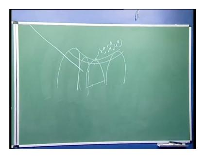
If you try to visualize the shape of the Lagrangian function in the x subspace, then at x star you will find then it has a minimum like this on the hand in lambda mu subspace it will have a maximum at that point that is means like this.
