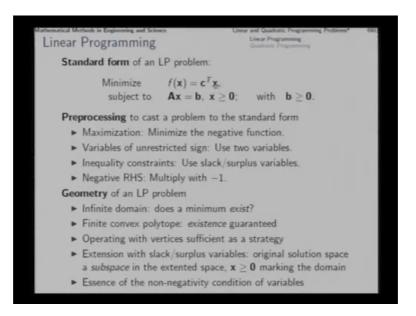
As you know a typical standard form of an LP problem is this minimize f x equal to c transpose x a linear function subject to a number of linear equality constraints with nonnegative variables x and nonnegative b. Now, if the original problem does not appear in this manner.
