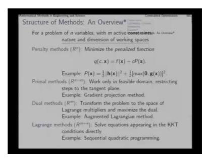
You can classify the different optimization algorithms different non-linear optimization algorithms into several classes into 4 classes depending upon the dimension of the space in which they conduct the search the simplest is the family of penalty methods in which the search is conducted in the same space in which the search would be conducted if it where unconstraint problems and constraints are included in the discussion in the search process through a penalty term like this.
