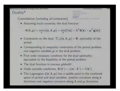
This is just for an over view if we assume local convexity that is near the solution point the function is convex in the x variables in the primal variables then the dual function is defined in this manner and constraints on the dual that is for the definition of the dual problem you will need this that is optimality of the primal.
