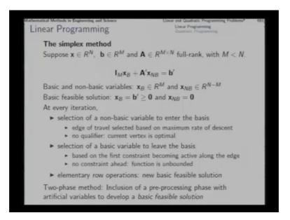
Now, in the simplest method what we do at every step we keep a set of basic variables that is equal to the number of linear constraints that we have and the other set of variables is taken as a non basic variables. Now, at every step we considered the variable having we considered only vertices to begin with and at every vertex quite if you constraints are on the active point right. So, those constraints which are active corresponding slag variable will be 0.
