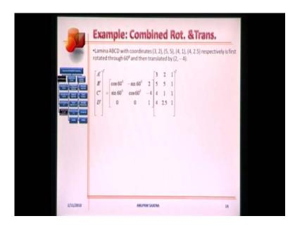
Let us take an example of combined rotation and translation. Lamina A B C D with coordinates of A as 3, 2, B as 5, 5, C as 4, 1, D as 4, 2.5 respectively is first rotated so 60 degrees and then translated by vector 2 minus 4. We can do the math, we know the results from the previous slide, this is the case of rotation and then translation. Once again I am performing translation on all the four points simultaneously here.
