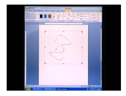
The second example feature design. Let me first draw a general curve here and then finally tends the positions of all these points. What this does is it allows me to change the local shapes of these curves. Many curves construes surface patches, so moving these points or transforming these points allows me to change the local shapes of those surface patches as well. I can go ahead and locally change the slope at a point. I will not be able to do feature design unless I perform transformations.
