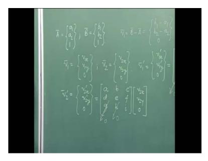
And let us say the coordinates of A, the homogenized coordinates A are a 1, a 2, 1 and those of B are b 1, b 2, 1. Notice that respect to some origin A and B will be position vectors. I vector algebra v 1 equals B minus A and a component form this is b 1 minus a 1, b 2 minus a 2 and 0. Notice this entry here for pre vectors this entry will be 0. Once
