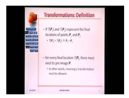
Let us say we have a point P and T of P represents the transformation of that point. If T of P 1 which is the transformed position of P 1 and T of P 2 which is the transformed position of P 2 represent the final locations of points P 1 and p 2. Then if T of P 1 equals T of P 2, then P 1 equals P 2 and the converse is also true that if P 1 equals P 2; then the respective images are the same. In other words for every final location T of P there must exist its pre-image P.
