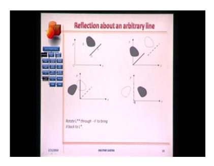
This is the operation; this line is rotated by an angle theta to coincide with the y-axis. Notice that the patch S has also been rotated accordingly. Step 3: Reflect S about the y-axis, graphically this picture defects the reflection. Next step rotate L double star through minus theta to bring it back to L star. In other words, I need to rotate this line to bring it back to this position like so.
