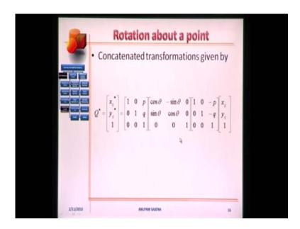
If we think about arranging different transformation matrices, again let me remind you that we are working with homogenous coordinates. x q star, y q star and 1 are the homogenous coordinates of the new location of Q, Q star and x q, y q, 1 are the homogenous coordinates of the previous location of Q. Of course, there are three matrices corresponding to three different transformations.
