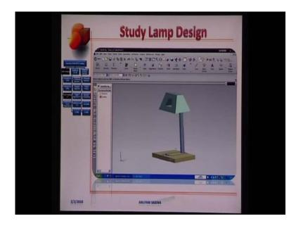
We can elongate the neck, if we want to get a new design. In a sense we are parametrically trying to change different geometric features of this design, without actually having to redesign the entire lamp from scratch and it is this feature, that is very nicely employed in complex solve modeling.
