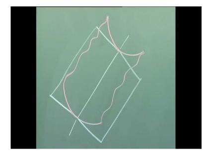
This is the common edge, this is the first face on the block, this the second face on the block, this would be third face on the cylinder and this would be the fourth face from this cylinder four faces.
