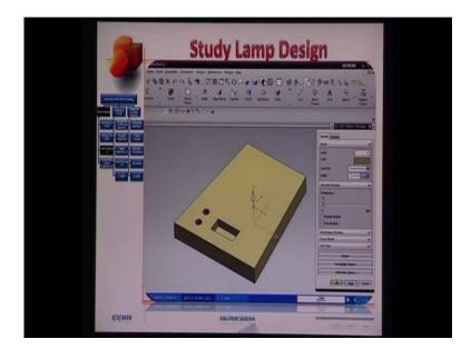
This is how we see different part holes. We can actually change the colors of different parts if we want. Next we will try to design a prismatic connector that connects the base to the powerful. We had this rectangular feature on the top phase of the base and we have this circle art. The idea is to get the connected again a prismatic shave, through this non-leaner speed; this rectangular cross section is going to be swept the along circle of art.
