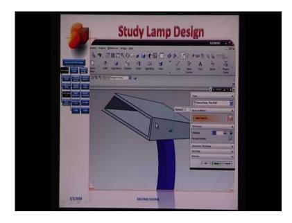
After we do that, we will introduce a shell like structure to represent the bulb holder; the thickness is about 1.5 units. We have a basic lamp design ready. These are different relations that Salish at used to design this lamp. By a metric solving modeling allows us to choose different features in the design and modified them locally. So that, we do not have to undergo the entire planes taking design procedure.
