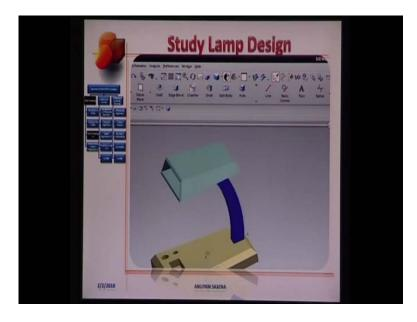
Let us now try to enlarge the base of the lamp and absorb how the design looks. We had different dimensions here, which are relating each other. If we change any one or two of these dimensions are base, we get a large this is one key feature of parametric solid model. We had to have relations between different features and face.
